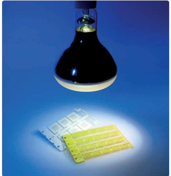
UV-light resistance testing
