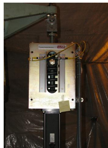
Exlar actuators have several advantages over hydraulic including higher energy efficiency, higher uptime from lower maintenance, repeatable performance, much smaller footprint and a less-costly infrastructure. Common process applications include inlet guide vanes, steam turbine governor valves, bypass valves and spray valves for the power industry as well as pipelines and isolation valves for the oil and gas industry.
