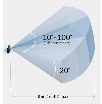
Aperture is field-selectable, and dynamically adjustable in 10° increments.
