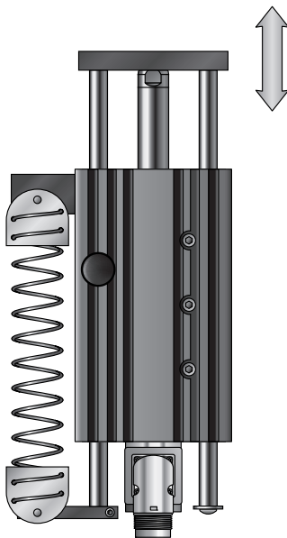
Weight compensation with mechanical spring
