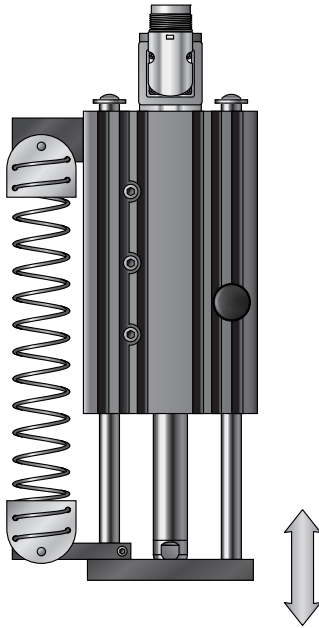
Weight compensation with mechanical spring
